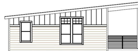
LEFT SIDE ELEVATION MONO-SLOPE ROOF SLOPED CEILING, LOW REAR TO HIGH FRONT (HITCH)
